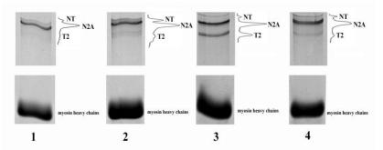
The changes in titin isoform composition in skeletal muscles of Mongolian gerbils under real microgravity conditions. Electrophoresis was performed in a vertical mini-gel containing 0.55% agarose and polyacrylamide 2.1-2.3%.
